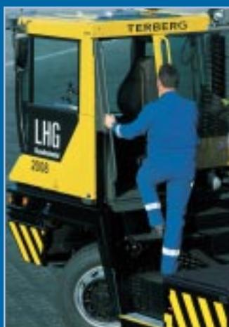
Standard feature: rear sliding door, provides safe and easy cab access from either side of the tractor.
