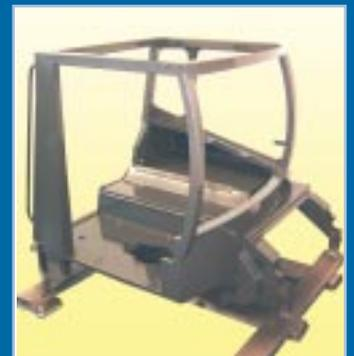
Strong, all steel cab structure (fully Fops & Rops tested), ensures maximum driver protection.
