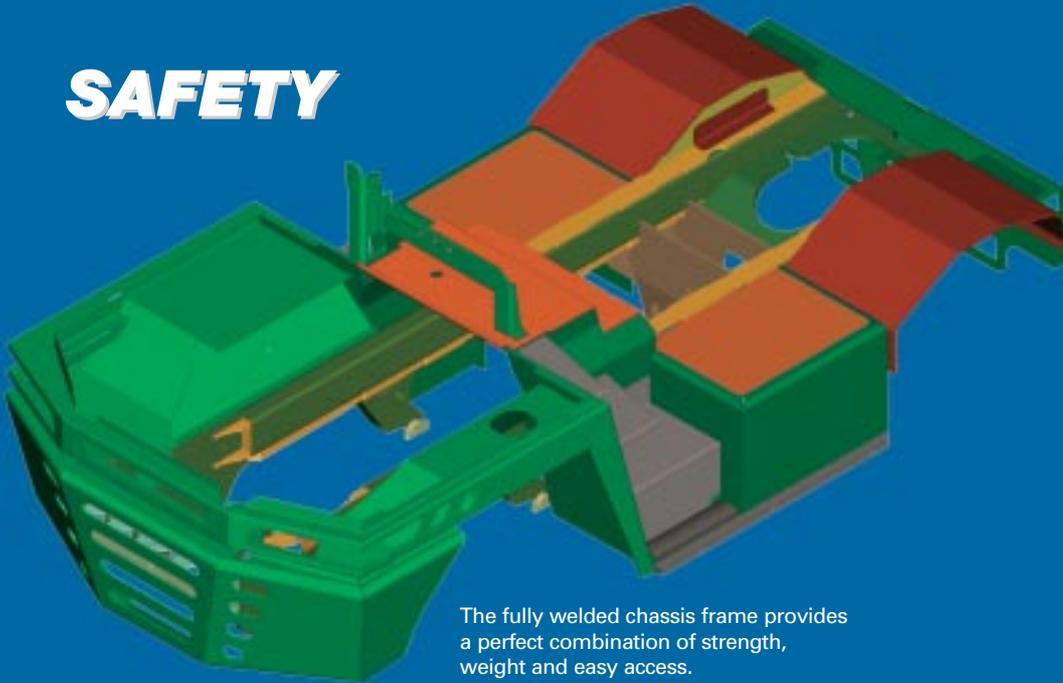
The fully welded chassis frame provides a perfect combination of strength, weight and easy access.
