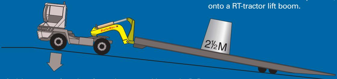
**RoRo tractor with SafeNeck:** A low centre of gravity + forward mount position on the RoRo tractor, enable the SafeNeck to transfer adequate load to the tractor front axle to improve overall stability. Use of the SafeNeck can increase the safe working capacity of a standard RoRo tractor by up to 250%.
