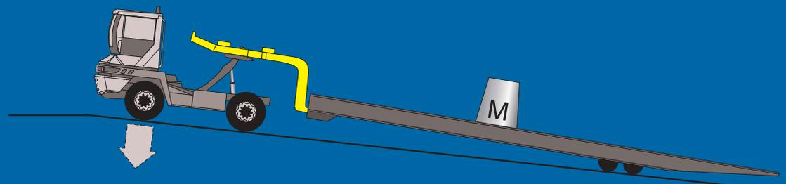
**RoRo tractor equipped with conventional gooseneck:** The standard location of a conventional gooseneck on a RoRo tractor + high centre of gravity during normal lift procedures whilst on a ship's ramp, will reduce weight distribution to the front axle - this affects and restricts the safe permissible payload capacity of the vehicle.
