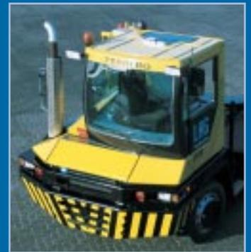
The cab is recessed well within the chassis frame, providing protection against damages.
